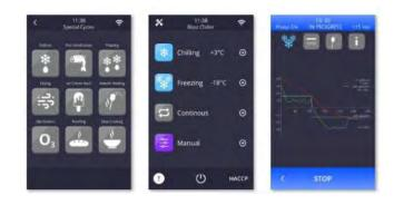
Touchscreen interface with 5" screen for a smart use of the machine. Multifunction and multilingual electronic board (8 languages). Customization of all parameters for each cycle: duration, ventilation level, temperature, etc. Possibility to create and save in your own recipe book the perfect cycles for the
