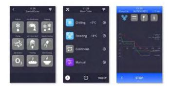
Touchscreen interface with 5" screen for a smart use of the machine. Multifunction and multilingual electronic board (8 languages). Customization of all parameters for each cycle: duration, ventilation level, temperature, etc.
