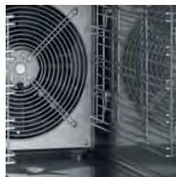
Detail of internal ventilation
